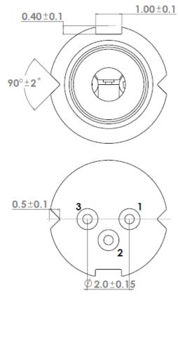
Note: Tolerance is  $\pm 0.05 \text{mm}$  for items without tolerance marking
