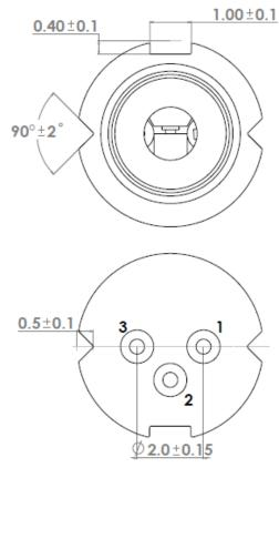
Note: Tolerance is  $\pm 0.05 \text{mm}$  for items without tolerance marking
