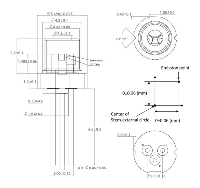
Note : Tolerance is  $\pm 0.05 mm$  for items without tolerance marking
